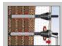
Step 8: adjust the depth of the MTH THERMAX as needed
