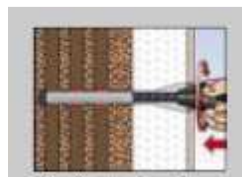
Step 7: manually install MTH THERMAX by turning
